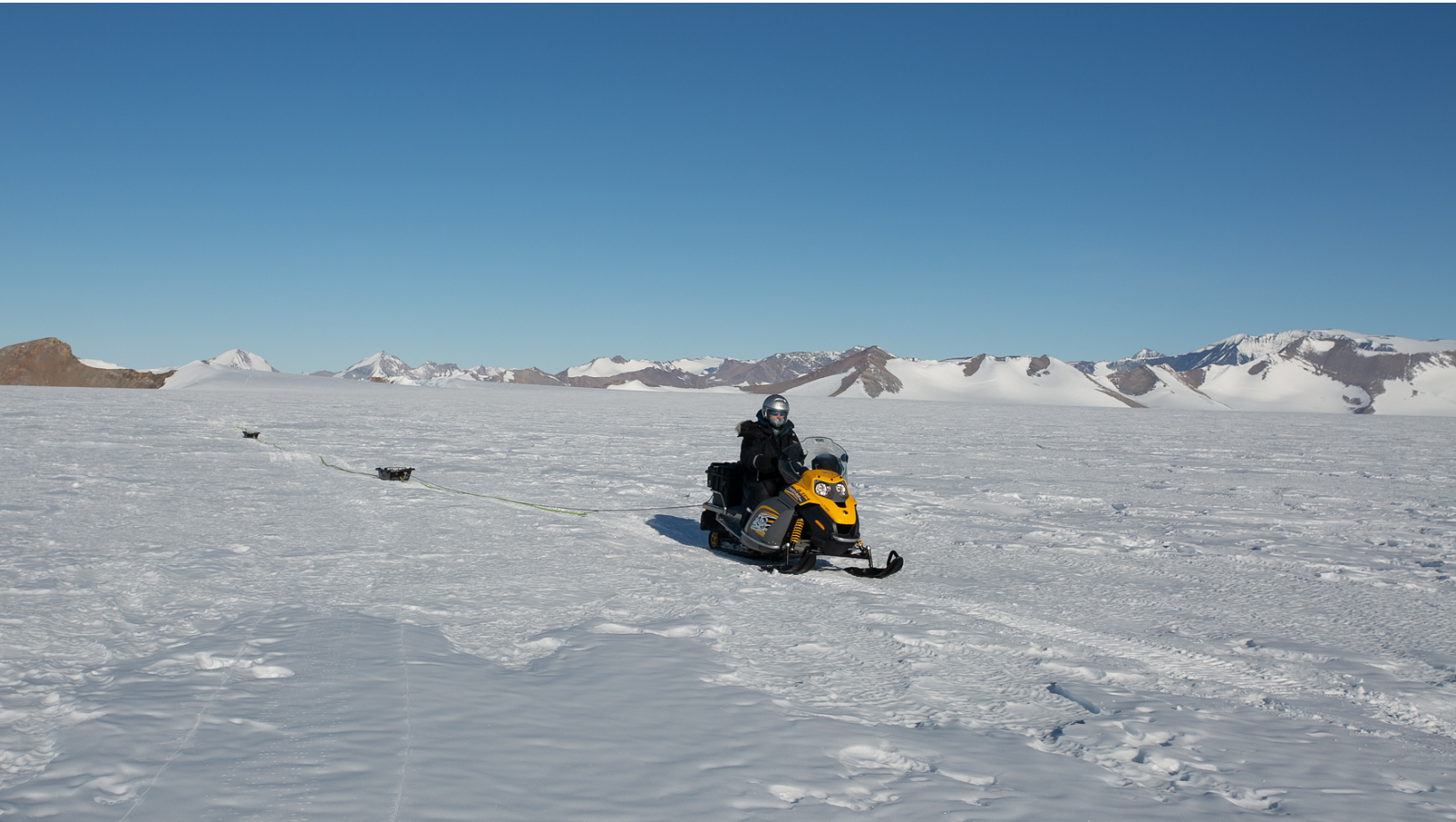
Dr Kate Winter undertaking a radar survey to identify subglacial lakes in Antarctica in 2020
