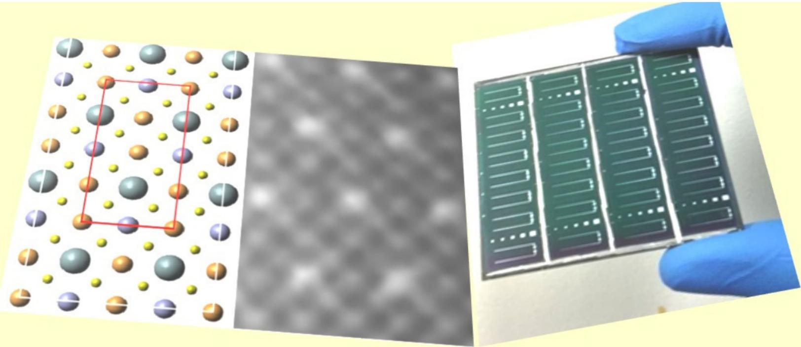
Our route to high-performance and scalable solar cells (right) is through understanding the relationship of solution-processing to the atomic-structural ordering and optoelectronic properties of the semiconducting-materials (left).
